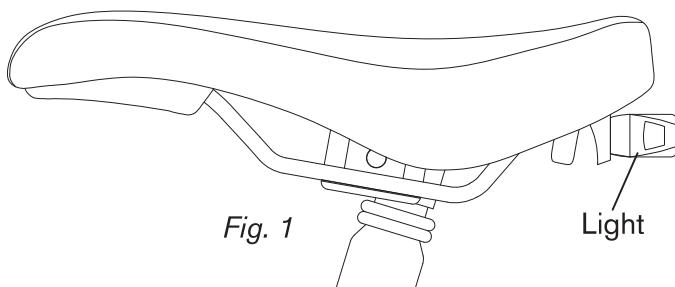
The Viz 150 light fits to a bracket, mounted to the rear underside of the saddle (fig. 1). The mounting point (fig. 2) was introduced onto the Brompton saddle midway through 2016, saddles produced before this time do not have the mount and are not compatible with the Viz 150 light.
