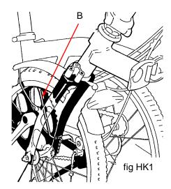
up too far, then a) it may catch on the spokes, and b) it may slide off the tube causing the bike to unfold inadvertently. will contact the tube CHS at C before has dropped to its fully folded position. chainwheel or (if fitted) the derailleur the front wheel spokes will clash with folded. If the hook is ineffective, and/or above in mind, judicious bending of the should cure the problem.
