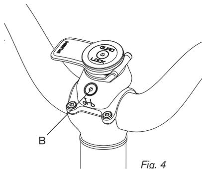
Install a Quad Lock compatible phone to the mount by holding it directly above the mount at a 45 degree angle, apply downward pressure and twist (in portrait orientation only on Mid Rise Handlebars).
