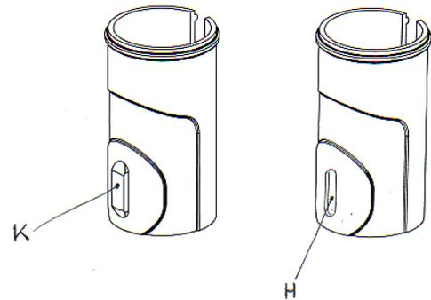
Prise out the existing sleeve. When you have removed the sleeve, you will be able to see whether there is a slot cut in the forward wall of the frame tube in which the sleeve sits: if this slot is present, then use the sleeve with the upstanding key as the replacement.
