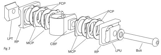
Refit the saddle to the Pentaclip and slide onto the seatpost, positioning it half way up the small diameter of the seatpost. Gently tighten the Pentaclip bolt with a 5mm hex key, leaving the assembly loose enough to adjust the saddle position. Ensure that you have the Pentaclip in the correct orientation and the saddle position and angle is correct. Once the saddle position is set, tighten the Pentaclip bolt to 15Nm.
