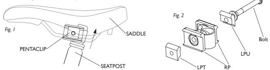
The Pentaclip can now be taken apart and the plates MCP and clamp band faces CBF degreased (fig. 3). Once the parts are clean and dry the Pentaclip can be reassembled with the clutch-plates fitted into the rail-plates (RP) in the order shown below. Plates MCP should be fitted with the formed 'ears' offset towards the outside of the bike (in order to engage fully with the rail-plates RP). The plates FCP may be a tight fit on the square splines.
