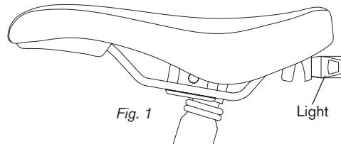
The Rapid Mini light fits to a bracket, mounted to the rear underside of the saddle (fig. 1). The mounting point (fig. 2) was introduced onto the Brompton saddle midway through 2016, saddles produced before this time do not have the mount and are not compatible with the Rapid Mini light.
